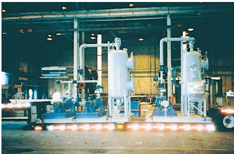
Two skid-mounted factory prepiped and wired recirculation/pressurization systems reduce site installation costs.
